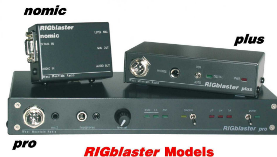
Figure 9. The RIGblaster computer / radio interface
